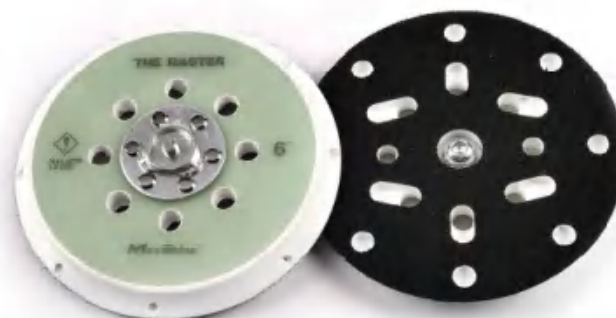
3011150P 6" (150mm) Max OPM: 12000 Thread: 5/16"-24 Hole: 8
