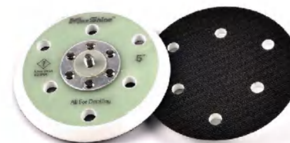
3013125 5" (125mm) Max OPM: 12000 Thread: 5/16"-24 Hole: 6
